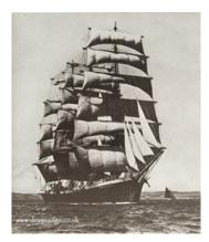
In the early 1800's, a new kind of ship was manufactured. It was a leaner, more slender ship, built for speed rather than capacity. Its sharp long prow was made out of expensive oak, and its sails spread 160 feet across. These ships were called clipper ships. They ran wide open, day and night, virtually ignorant of weather conditions, arriving beaten and battered at their destination, but on time no less.
